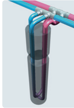
Installation of pipe loops crosswise
